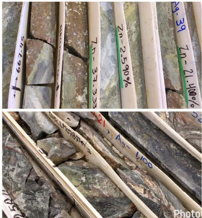
Top: High-grade zinc drill core from Southern Silver Exploration's shallowly dipping Blind Shoulder zone, a skarn target at roughly 600 metres depth. Bottom: High-grade silver drill core from the steeply-dipping Blind skarn deposit. Photos by Lesley Stokes.
